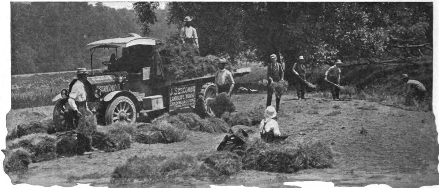
Peerless 3-ton truck used by J. Sercombe, a landscape gardener of Toronto, Ont. He has found that the motor truck is practicable for use in fields and on soft ground
